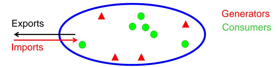
Balancing group: entity in a control area of an electricity system; it has to ensure that at every moment demand and supply is balanced
