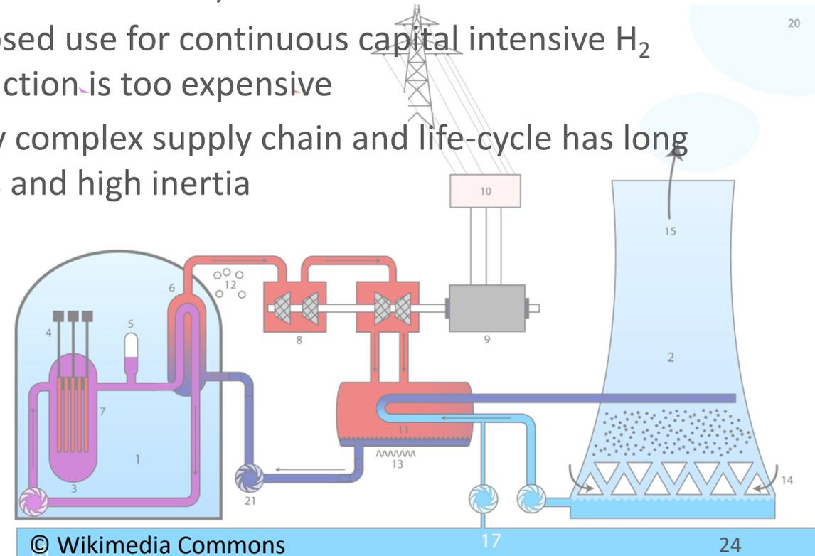
**Nuclear energy harvesting needs huge ancillary systems for fuel provision, safety, radiation protection, low-efficiency energy conversions (heat → mechanical energy → electricity) and waste disposal**
